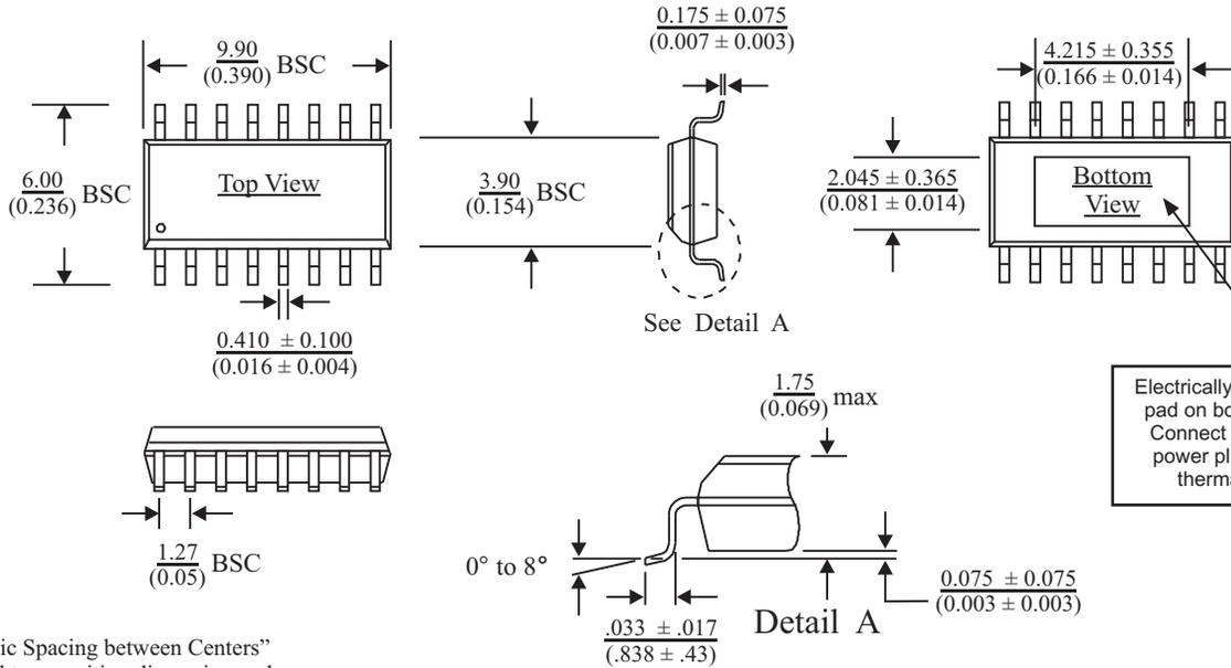
Electrically isolated heat sink pad on bottom of package. Connect to any ground or power plane for optimum thermal dissipation.
