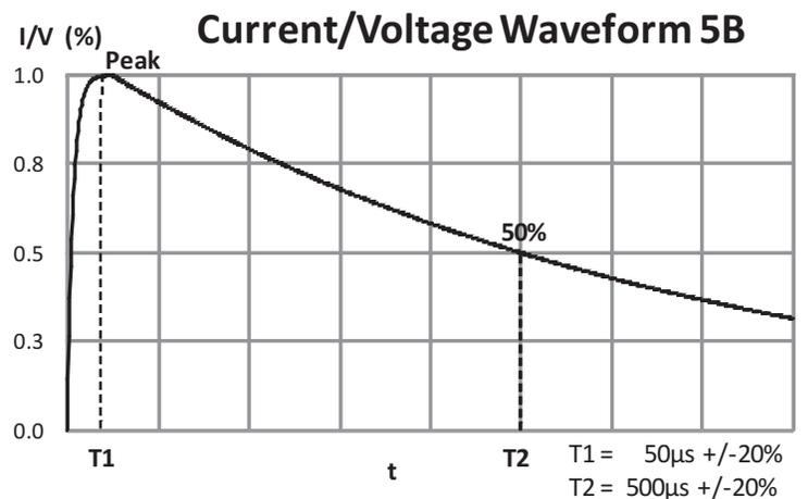
Figure 12. Lightning Waveforms
