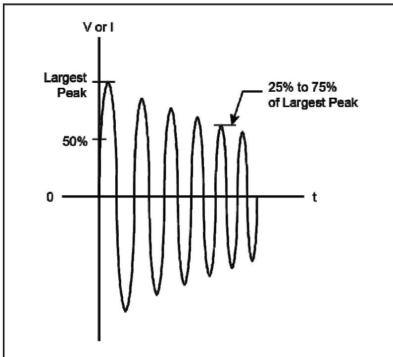
Figure 5. DO-160G Lightning Induced Transient Voltage Waveform 3.
