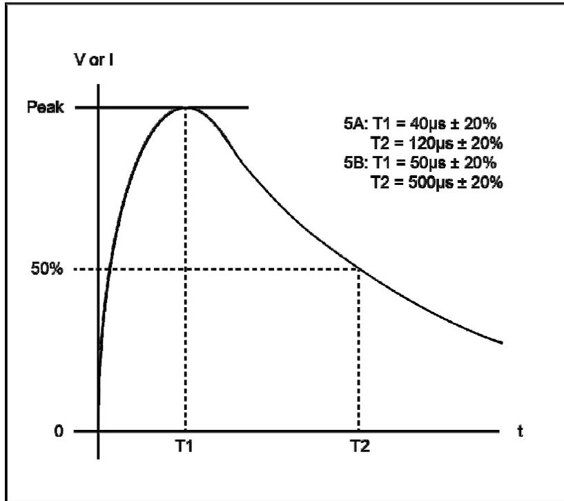
Figure 6. DO-160G Lightning Induced Transient Voltage Waveforms 5A and 5B.
