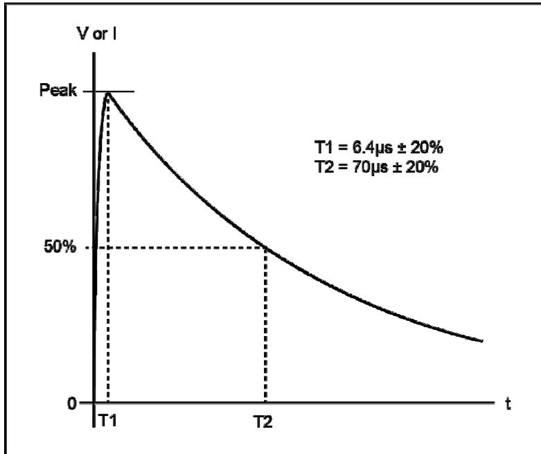
Figure 6. DO-160G Lightning Induced Transient Voltage Waveform 4.
