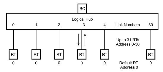
Remote terminals based on the Holt HI-6140 protocol chip and HI-4853 transceiver for RS-485 can perform all three modes defined in SAE AS5652: Spec Mode, Switch Mode and Link Mode.
