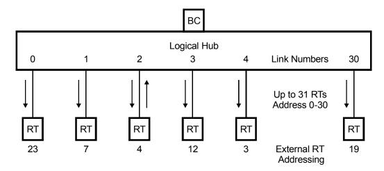
In Spec Mode, the Logical Hub does not know in advance which Hub-RT link will carry the RT response. The Logical Hub must be prepared to route a response from any RT link to the Bus Controller. In the most likely scenario, the Hub logically-ORs received data from all connected RS-485 Hub-RT transceivers.
