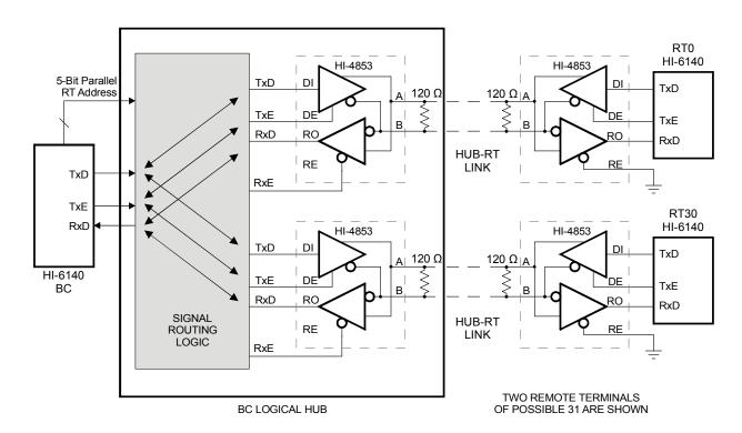
Backing off on the signal interface detail and showing other BC and Logical Hub considerations results in the diagram below. The 5-bit parallel RT address output is enabled when the Bus Controller HI-6140 is configured with register 0x4D bit 3 set to logic 1.
