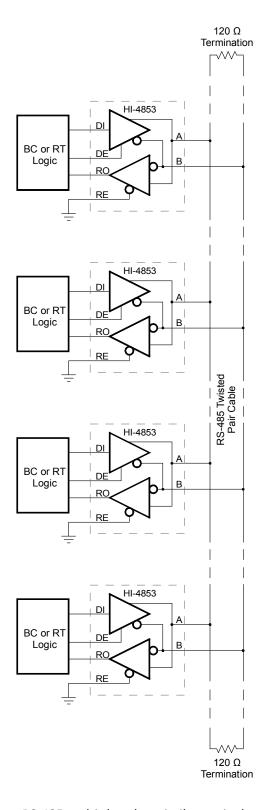
Conventional 10 MB/sec RS-485 multi-drop bus similar to single-cable MIL-STD-1553. No known network standard applies this approach, but it is functional when each "BC or RT Logic" represents a HI-6140 protocol IC.
