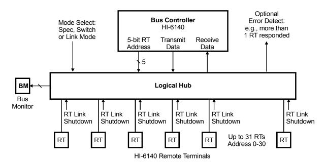
The unique addressing scheme for Link Mode is selected when register 0x4D bit 4 is set to logic 1. So configured, the 5-bit parallel RT address output specifies the RT address derived from the BC Instruction List, but each Command Word issued by the Bus Controller contains embedded RT address 00000 at Command Word bits 15:11. Please refer to the HI-6130 data sheet for BC Instruction List setup.
