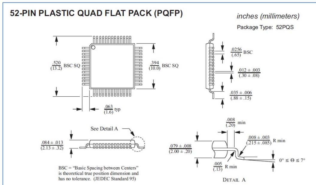
Figure 2) (GREATEK & MILLENNIUM MICROTECH –MQFP)
